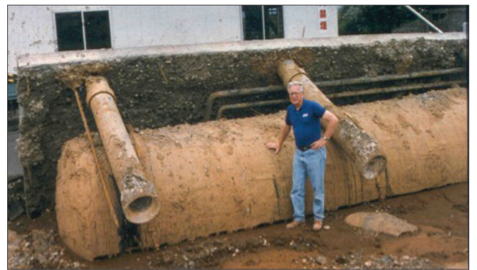
Figure 18. Buried oil storage tank at an industrial facility that floated to ground surface due to liquefaction of subsurface soils during the 1993 Hokkaido-nansei-oki, Japan earthquake. 24
